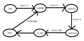
Fig: 10. State machine of ADC to DAC
